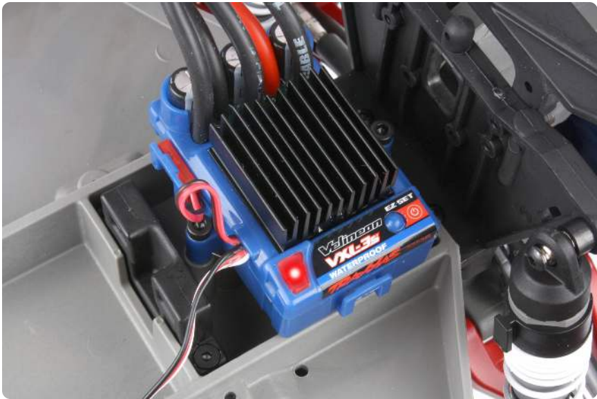
The VXL-3s speed control. This is the box that lets a 3S pack into the truck.
